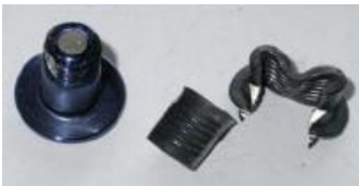
SLFC-MV collars cut with FCMV hydraulic cutter
